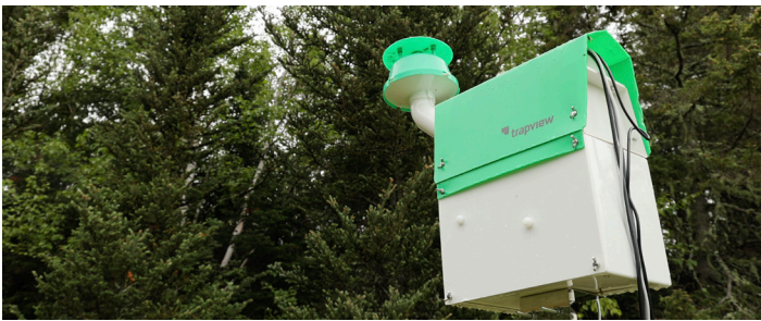
Automated spruce budworm trap, New Canada, Maine.
